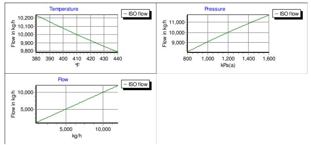
The charts of interest are Temperature and Pressure. The chart for flow is of no interest since it only displays flow calculated by FlowCalc32 versus flow calculated by FlowCalc32, which is a straight line. In the other two charts you can see the flow calculated by FlowCalc32 when the temperature and pressure changes. Note that in the reference point (temperature = 410 F and pressure = 1200 kPa) the flow is 10000 Kg/h, which is
