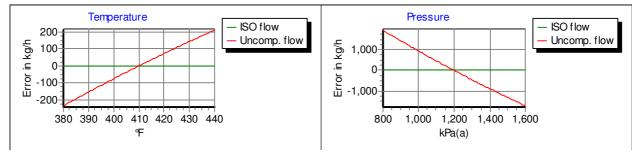
In these charts you can see that the flow calculated by FlowCalc32 (ISO flow) results in an error of 0 kg/h regardless of changes in temperature and pressure. The reason for this is that the error is defined as the difference of the flow calculated by a flow formula and the flow calculated by FlowCalc32s flow formulas. The uncompensated flow on the other hand shows relatively large errors as expected.
