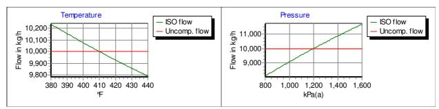
As you can see in the charts above the uncompensated flow is constant at a level of 10000 kg/h. This is the flow in the reference point and since the uncompensated formula doesn't compensate for changes in temperature and pressure the flow graph is only a straight line at this level.
