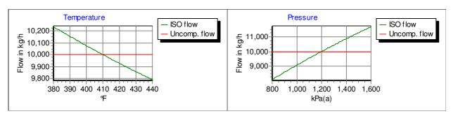
As you can see in the charts above the uncompensated flow is constant at a level of 10000 kg/h. This is the flow in the reference point and since the uncompensated formula doesn't compensate for changes in temperature and pressure the flow graph is only a straight line at this level.
