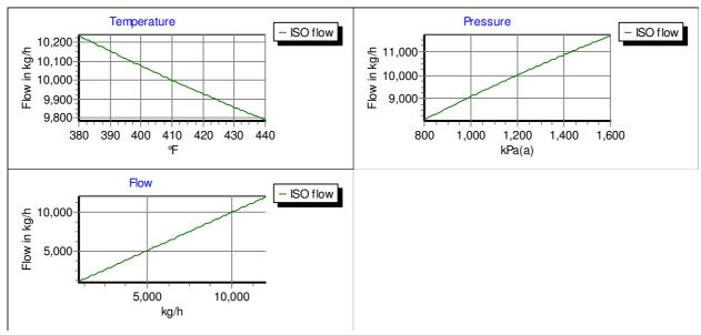
The charts of interest are Temperature and Pressure. The chart for flow is of no interest since it only displays flow calculated by FlowCalc32 versus flow calculated by FlowCalc32, which is a straight line. In the other two charts you can see the flow calculated by FlowCalc32 when the temperature and pressure changes.
