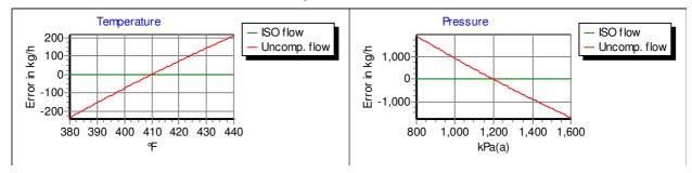
In these charts you can see that the flow calculated by FlowCalc32 (ISO flow) results in an error of 0 kg/h regardless of changes in temperature and pressure. The reason for this is that the error is defined as the difference of the flow calculated by a flow formula and the flow calculated by FlowCalc32s flow formulas. The uncompensated flow on the other hand shows relatively large errors as expected.
