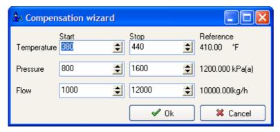
In this window you can set the parameter span in which the compensation wizard will try to find an optimal flow formula. In our case we don't have to change the limits so we proceed by clicking "Ok"
